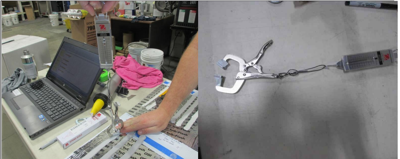
Photos: (left) pull test in process, (right) scale with clamp.
